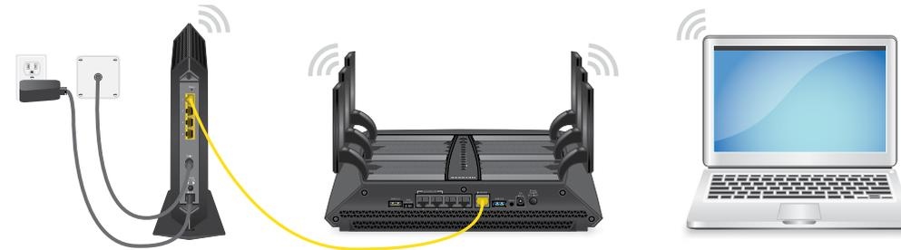
1. Reboot the cable modem by unplugging the power cable from the cable modem and plugging it back in.
