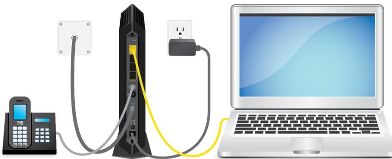
**Figure 5. Connect your cable modem to a computer**
